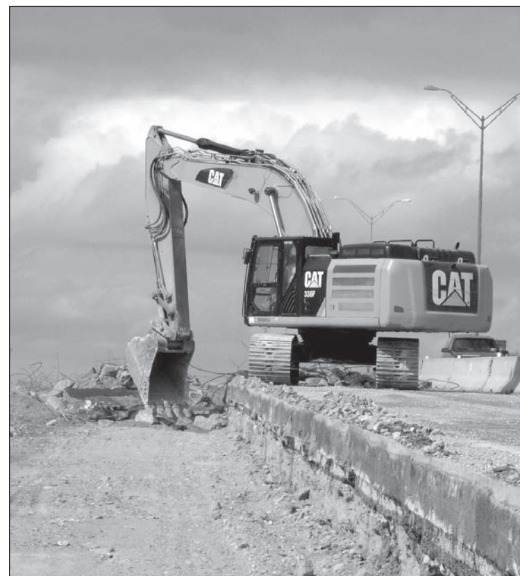
BIG MOVER – The Caterpillar 336F Excavator weighs 88,400 lbs. – depending on the configuration and attachments. It burns about 8 gallons of deisel an hour. The boom can reach out 38.7 feet on level ground and the bucket can hold an impressive 70.5 cubic feet of material.
